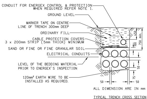
1. INSTALL A NEW COMMUNICATIONS CONDUIT OF MINIMUM SIZE, 100mm LD PVC WHITE CONDUIT.
