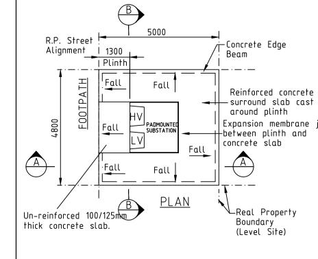
1. Backfill excavated area with crusher dust deco or pit sand and compact in place. Ensuring that only pit 2. Reinforced concrete surround slab:
