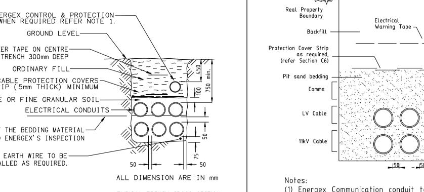
(1) Energex Communication conduit to be 100mm white located top
